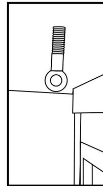
3. Slide the supplied metal cable in to one side of the metal crimp lock. Thread the cable through the Roof Anchor eye hook then through the other side of the metal crimp lock. Crimp the Crimp Lock using pliers to secure the cable in place. Secure this with the cable lock supplied.
