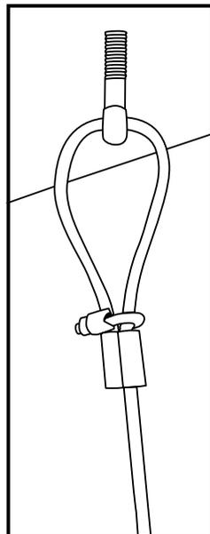
4. Repeat section 3 above with the other end of the metal cable securing it to the J bolt ground anchor. Be sure the cable is pulled tight.
